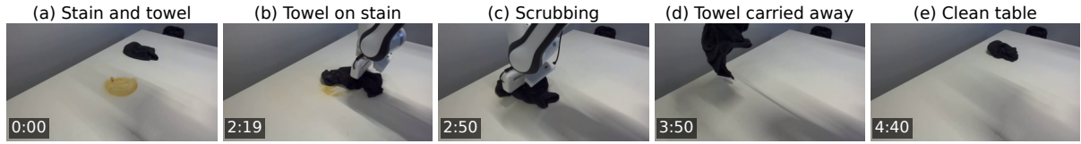
Figure 28 | Wiping a stain, trial 7b , from the left exterior camera. (a) The poured stain and the towel heap; (b) the grasped wad pressed on the stain; (c) scrubbing; (d) the towel is carried back; (e) the table after one pass. Time is from the first frame.
