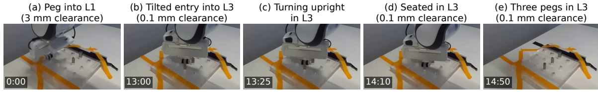
Figure 31 | The ManipulationNet peg-in-hole challenge , final run, from a crop of the left exterior camera. (a) A peg inserted into L1 (3 mm clearance); (b)–(d) the rectangle peg entering L3 (0.1 mm clearance) corner first, turned upright, and seated; (e) the three pegs seated in L3. Time is from the first frame.
