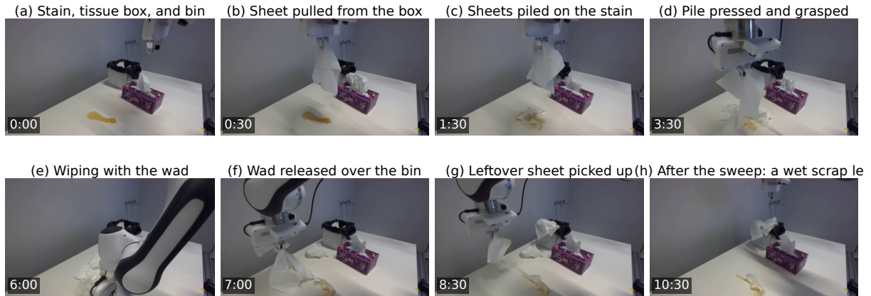
Figure 29 | Wiping with paper towels, second wet run , from the left exterior camera. (a) The poured stain, the tissue box, and the bin behind it; (b) a sheet pulled from the box; (c) six sheets piled on the stain; (d) the pile pressed and grasped as a wad; (e) wiping, with the towel program’s zig-zag; (f) the wad released over the bin; (g) a leftover sheet picked up by the sweep; (h) the table afterwards, with a flat wet scrap the sweep missed. Time is from the first frame.
